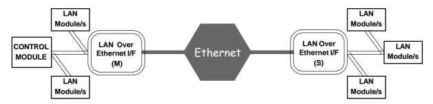
Up to 4 Slave units can be connected to the Ethernet network to connect the Control Module RS485 LAN to one or more other Modules in a number of remote locations.
