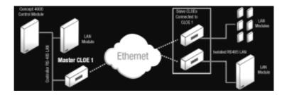
An interface consists of a Master and up to 4 Slaves. The CLOE boards are Installer configurable to be a Master or a Slave and employ 128-bit AES encryption for secure Ethernet communications.
