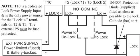
Heavy duty Fig. 8 cable (24/0.20 or 14/0.20) recommended for all Power & Lock wiring.
