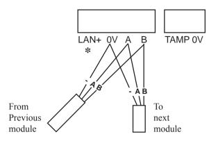
\* Note: If required, the LAN to subsequent Modules may derive +12V from "LAN+" or the incoming LAN cable.
