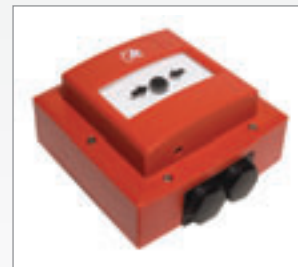
© EURVC-MCP-IP67 Conventional Eurotech Waterproof Manual Call Point Manual call point (IP67) for fast response manual operation of fire alarm system. Part No: 100-1011 Standard: EN54-11:2000 + A1:2005 Operating voltage: 20-38v Operating current: Ialarm: 50mA @24v
