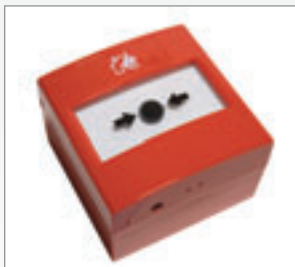
© EURVC-MCP-IP24 Conventional Eurotech Manual Call Point Manual call point (IP24) for fast response manual operation of fire alarm system. Part No: 100-1010 Standard: EN54-11:2000 +A1:2005 Operating voltage: 20-38v Operating current: Ialarm: 50mA @24v
