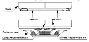
Fig. 2: Fitting the detector to the base
