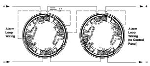
Fig. 1: Base wiring connections
