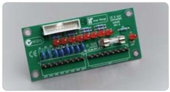
This handy expansion board complements the two on-board auxiliary outputs on the Concept 4000 Control Module with the addition of eight open-collector outputs. The board connects directly onto the Control Module.
